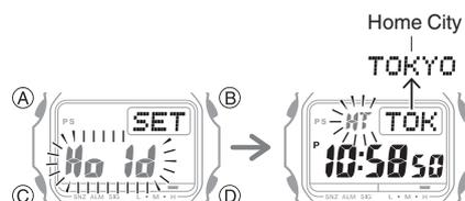
3. Keep pressing (C) until the setting you want to change is flashing.
