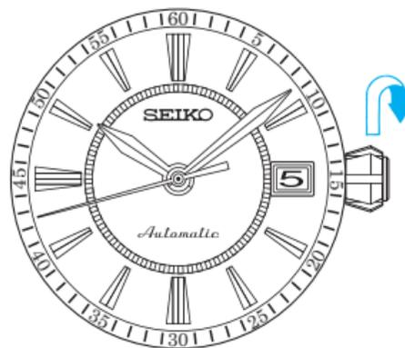
1. Slowly turn the crown clockwise (in the 12 o'clock direction) to wind the mainspring.
