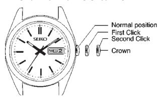
Gently pull the crown out as far as it will go. The watch will not run when the crown is in this "set" position. If the watch has a "screwdown locking crown," you may have to "unlock" it before you can pull the crown out. To do this, rotate the crown counter-clockwise (toward the bottom of the watch.) This unlocks the crown. Once it is unlocked, gently pull the crown out as far as it will go.
