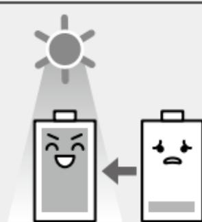
**This watch has a rechargeable cell which is charged by exposing the dial to light.**
