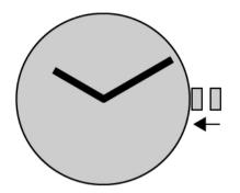
Press the crown back into its "zero" position near the base of the watch.
