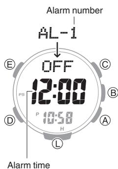
3. Hold down (E) for at least two seconds. Release the button when the hour setting starts to flash.
