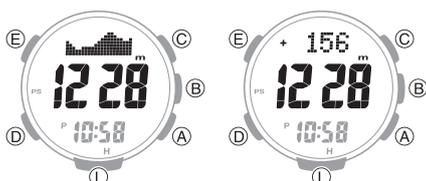
Entering the Altitude Mode will start altitude measurement and display the altitude at your current location.
