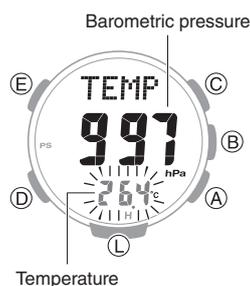
3. Press (D) to select the temperature correction or barometric pressure correction screen.
