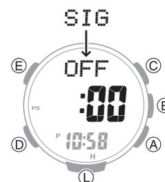
3. Press (B) to toggle the hourly time signal between enabled and disabled.
