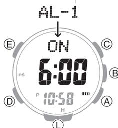
3. Press (B) to turn off the displayed alarm or the hourly time signal.
