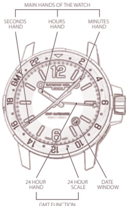
The **Nabucco** GMT bezel is marked with a 24 hour scale. This enables a second time zone display which can be read from the 24 hour hand.
